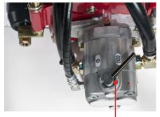
Reel Motor shut-off valve
